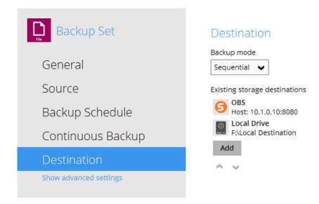
In the above example, data will first be uploaded to the OBS backup destination. When the upload is completed, data will be uploaded to the Local Drive backup destination.
