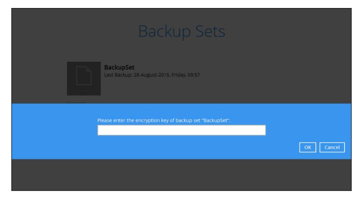
Answer) The client application will prompt for the encryption key of all existing backup sets when the user, if it cannot detect the present of the settings.sys file (within the operating system profile (e.g. ~/.obm/config/settings.sys).
