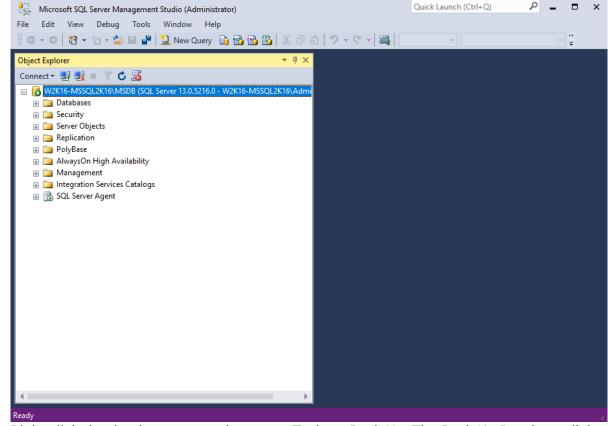
4. Right click the database name, then go to Tasks > Back Up. The Back Up Database dialog box shows.
