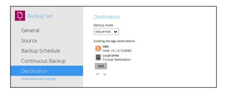
In the above example, data will first be uploaded to the OBS backup destination. When the upload is completed, data will be uploaded to the Local Drive backup destination.
